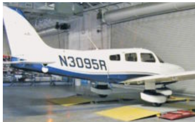
Figure 4-12. Weighing a Piper Archer using electronic platform scales.
