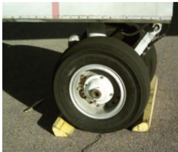
Figure 11-12. Wheels chocked fore and aft.
