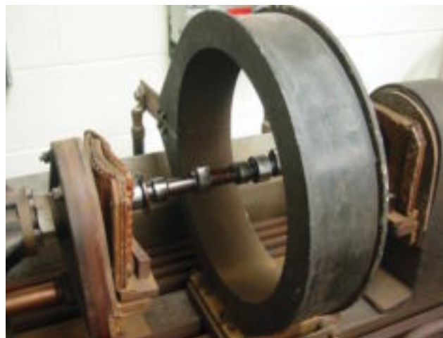
Figure 8-17. Longitudinal magnetization of crankshaft (solenoid method).
