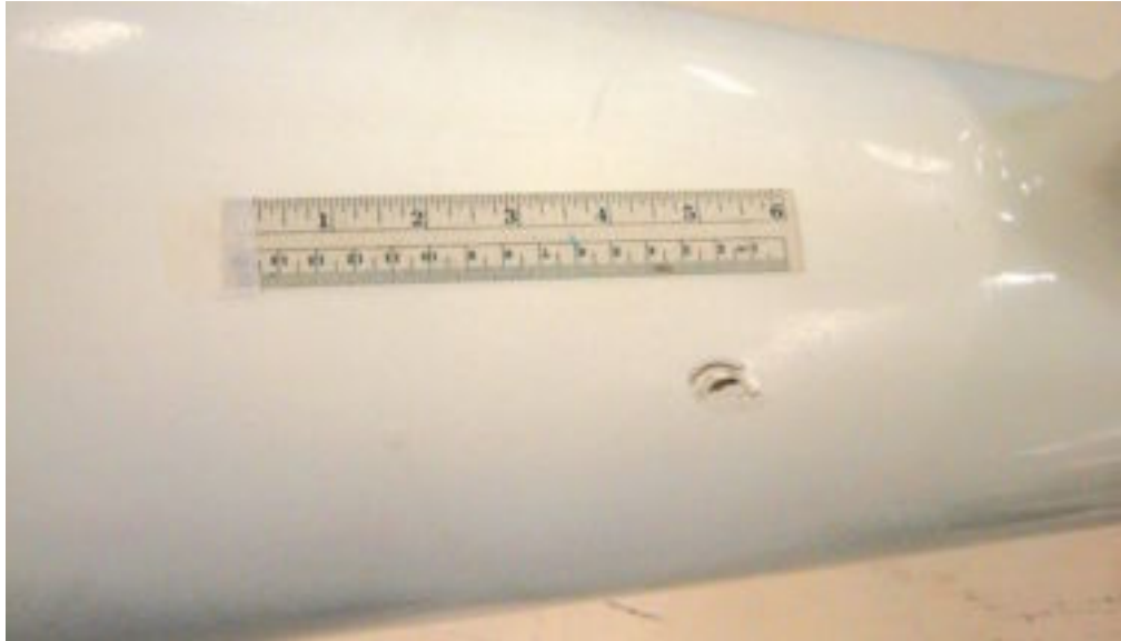
Figure 2-32. Digital image of impact damage.
