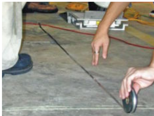
Figure 4-18. Measuring the nosewheel arm on a Cessna 310.
