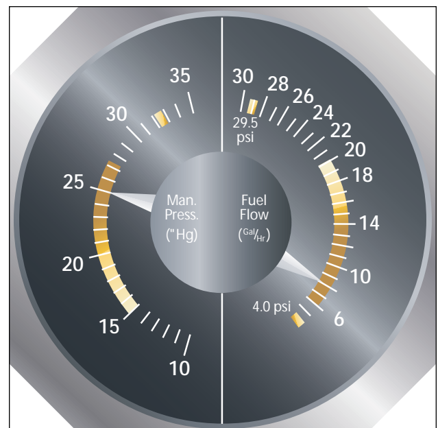
Figure 3-35. Manifold pressure gauge indicating absolute pressure.
