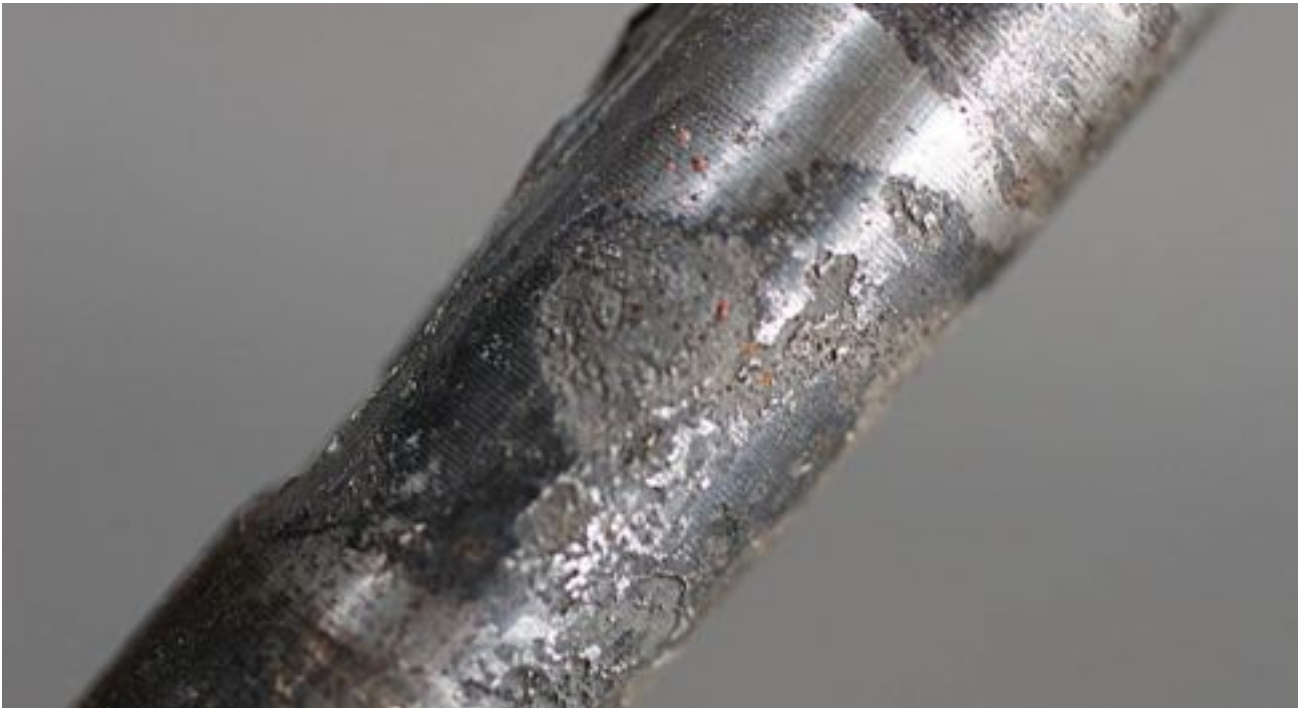
Figure 6-7. Dissimilar metal corrosion.
