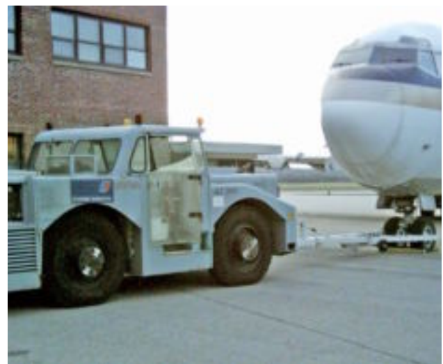
Figure 11-19. Example of a tow tractor.
