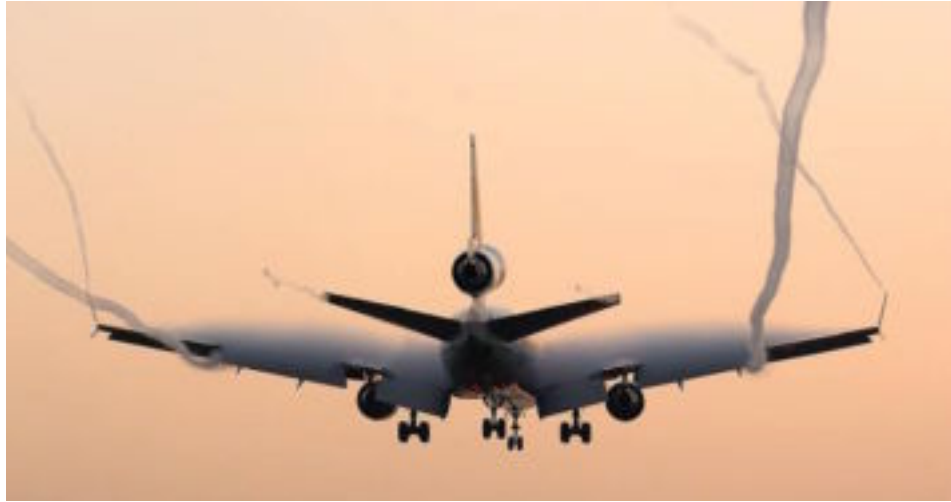
Figure 3-59. Wing and horizontal stabilizer vortices on an MD-11.
