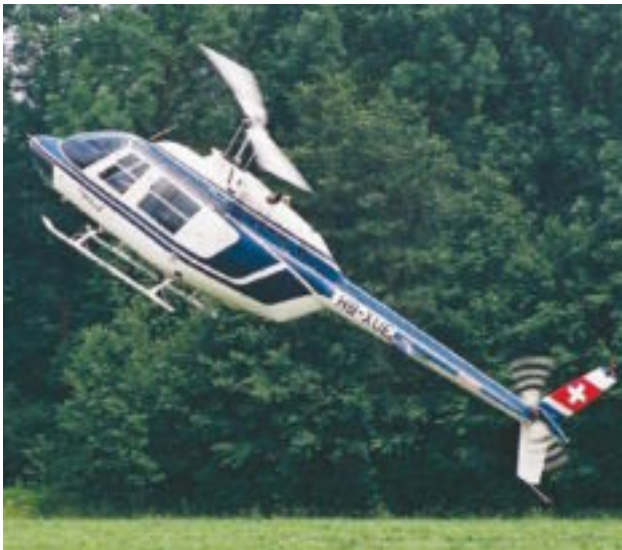
Figure 3-96. Bell Jet Ranger in final stage of autorotation.
