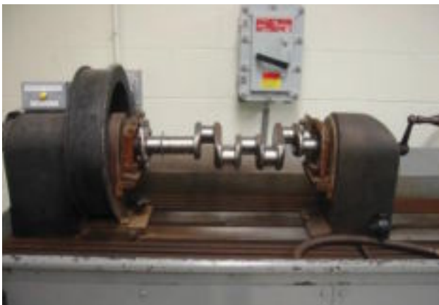
Figure 8-16. Circular magnetization of a camshaft.
