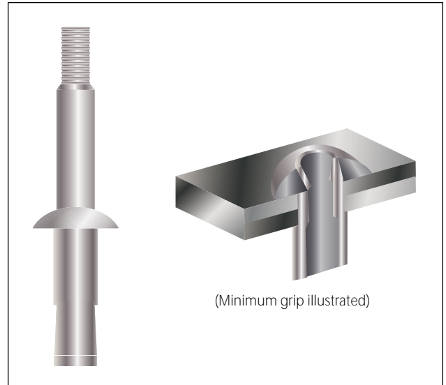
Figure 5-44. Wiredraw cherrylock rivet.
