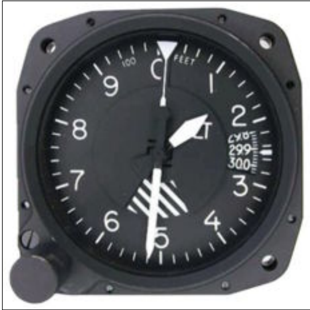
Figure 3-51. An airplane's altimeter is an aneroid barometer.
