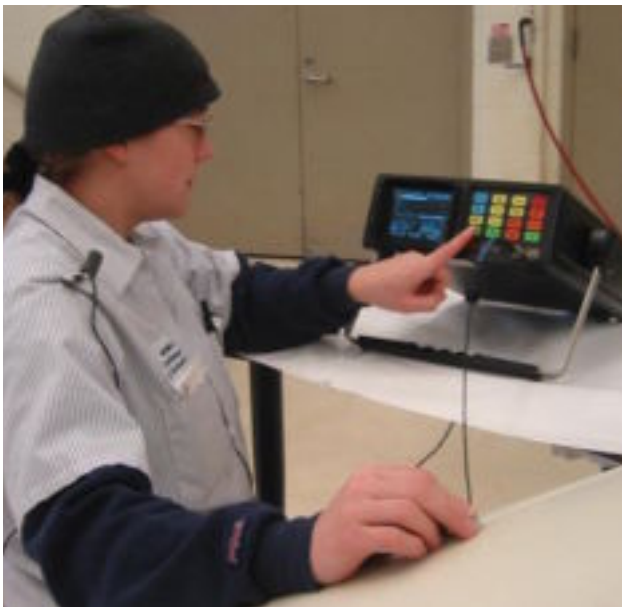
Figure 8-12. Ultrasonic inspection of a composite structure.
