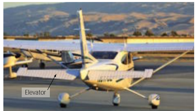
Figure 3-65. Elevator on a Cessna 182 provides pitch control.
