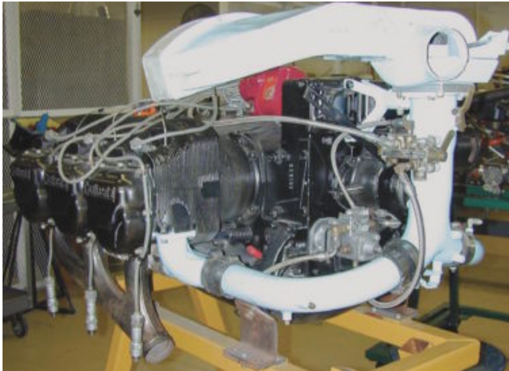
Figure 3-29. Aircraft piston engine cooled by convection.
