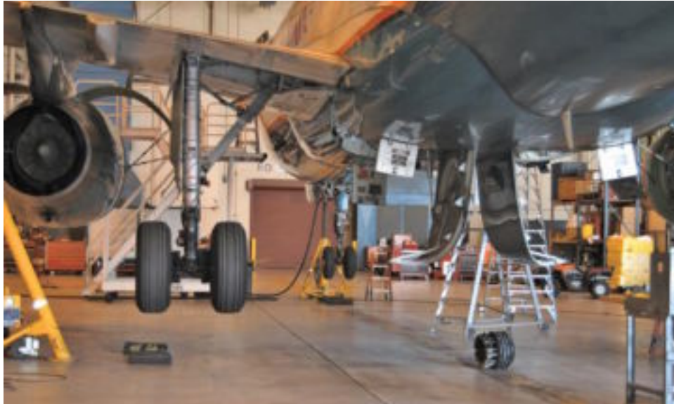
Figure 3-4. Airbus A-320 being jacked.
