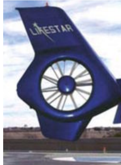
Figure 3-87. Fenestron on a Eurocopter Model 135.
