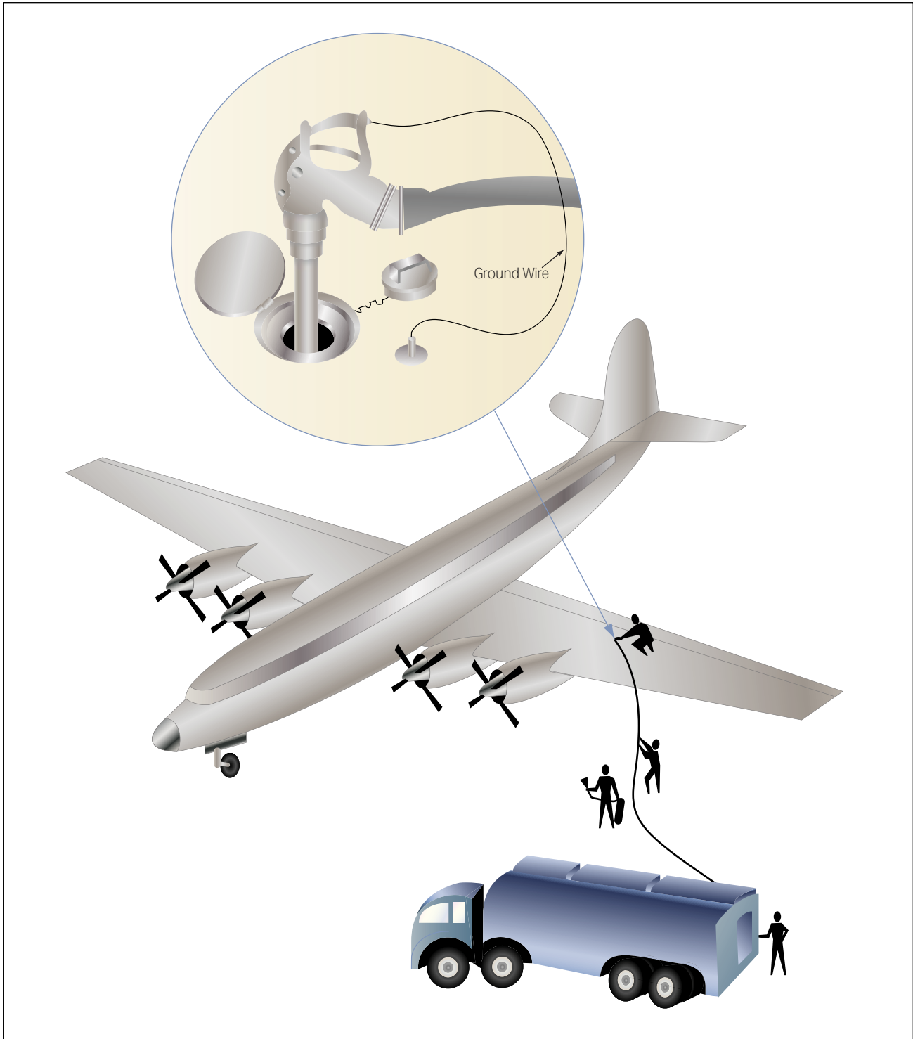
Figure 11-31. Refueling an aircraft by the over-the-wing method.
