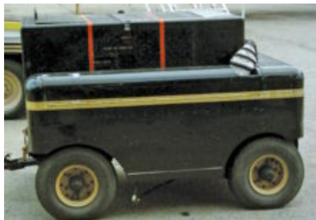
Figure 11-30. A portable compressed air cart.
