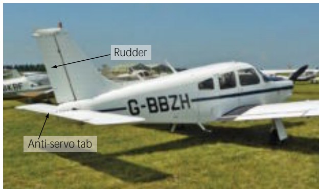
Figure 3-70. Rudder on a Piper Cherokee Arrow.
