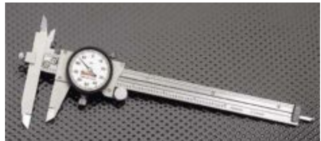
Figure 9-41. Electronic and dial indicator slide calipers.
