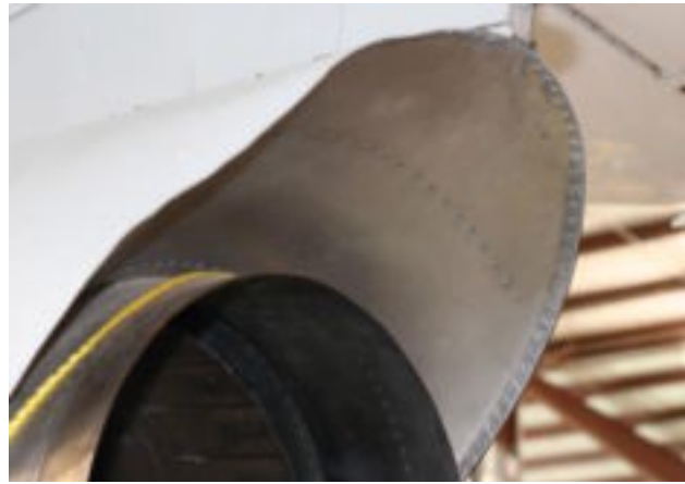
Figure 6-11. Exhaust nozzle area.
