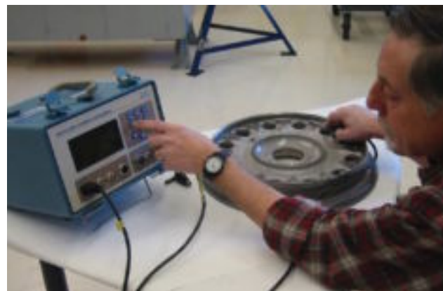
Figure 8-5. Eddy current inspection of wheel half.
